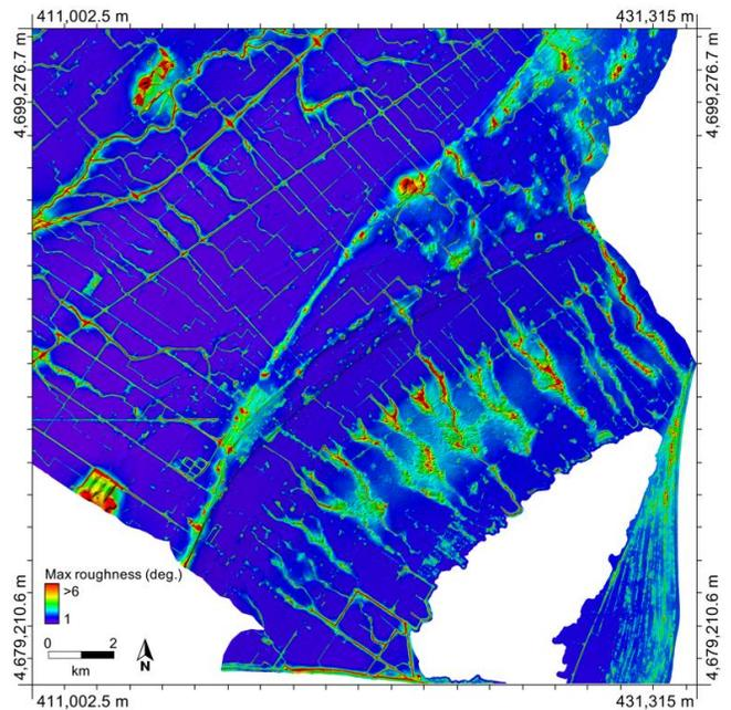
Figure 3. Maximum surface roughness (degrees) measured with filter sizes ranging from 3 to 5000 cells.
