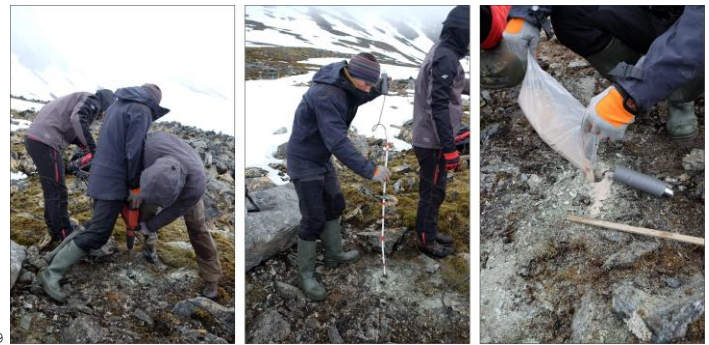
Figure 2. Installation of 1.5 m long thermistors string connected to mini datalogger (site TM13, see in Fig. 1, photographs: P. Tábořík).
