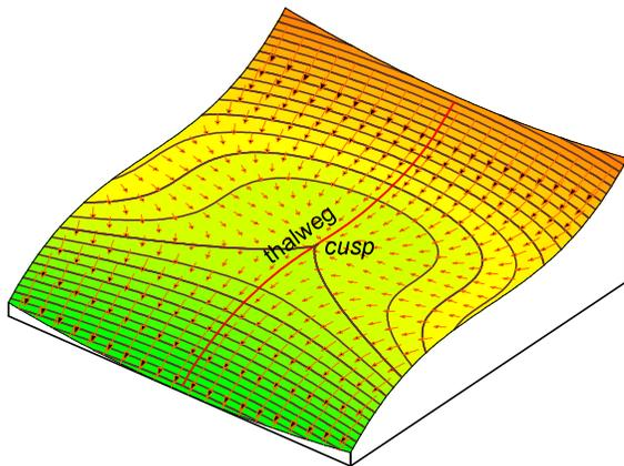
Figure 1. Remnant of terrace surface ( $z = x^3 + y^2$ )
