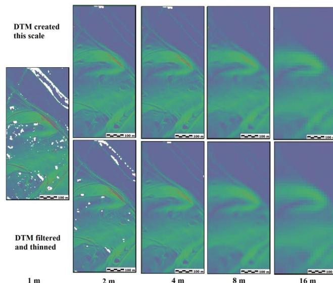
Figure 6. Effect of DTM grid size on computed slope maps, comparing two methods of creating the pyramid of grids.
