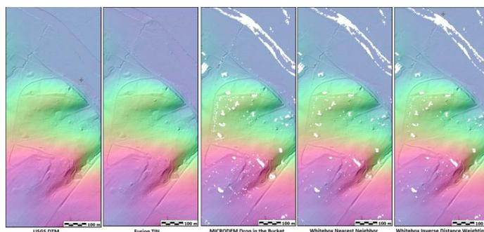
Figure 5. DTMs derived with differing interpolation algorithms.
