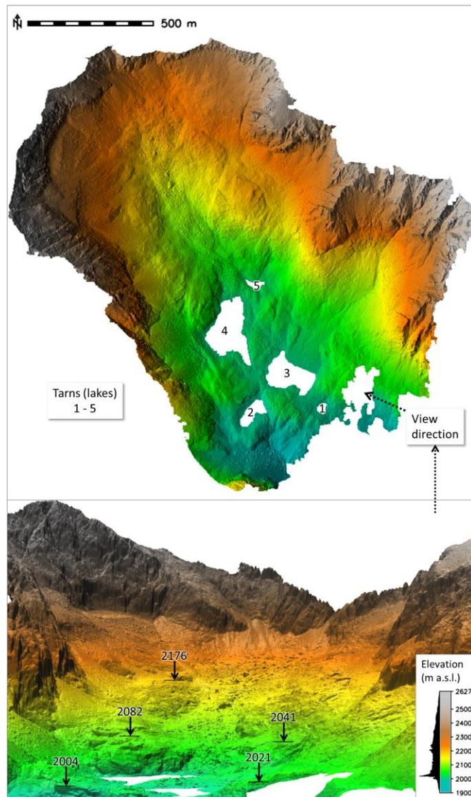
Figure 4. Final raster DEM (0.5x0.5 m cell size) resulting from a combination of TLS and UAV point clouds. Perspective 3-D view of the DEM is similar to that of Fig. 2. The values refer to local maxima altitudes of glacially polished bedrock. The areas of lakes 1-5 (tarns) are masked out.
